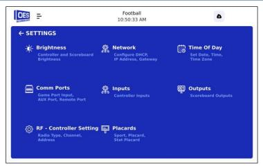
Touch the intended button on the **SETTINGS SCREEN** to adjust settings. The password for the SETTINGS SCREEN is **5833**.
