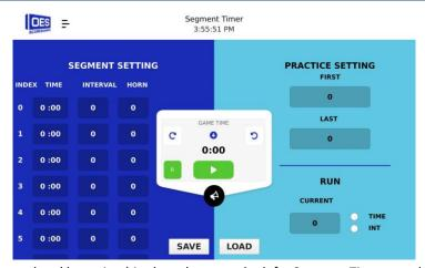
Enter the Segment time (and interval and horn time) in the column on the left. Segment Timers can be saved. Enter the first and last segment number on the right and press start or use the game remote to start the segment timer running.
